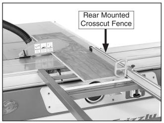
Figure 58. Crosscutting smaller panels.
